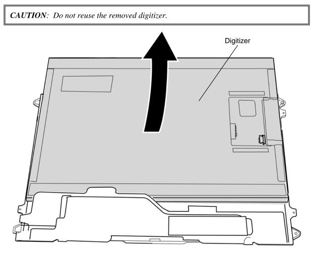
Figure 4-55 Removing the digitizer
